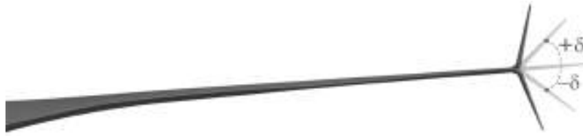
Figure 2: Active winglet principle with variable cant angle.
