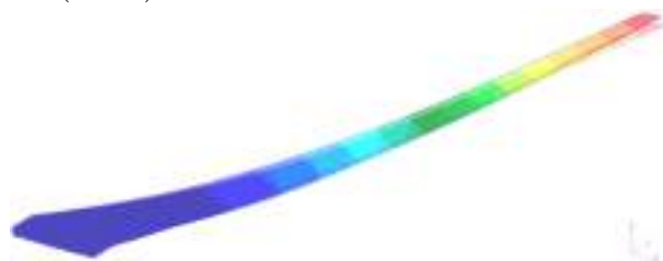
(b) Comparison of deformations of uCRM-13.5 wing for HF case (up) and LF case (down).
