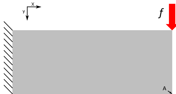
Figure 13: Cantilever beam system where The left boundary is fixed and the force is shown by the red arrow f . The point at which the displacement will be evaluated is labelled A.
