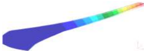
(a) Comparison of deformations of uCRM-9.0 wing for HF case (up) and LF case (down).
