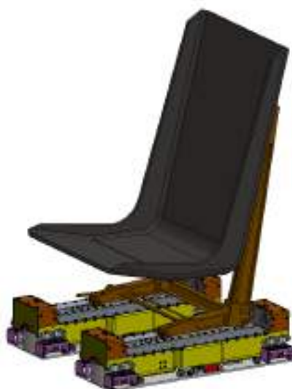
Figure 9 Bell-412 seat frame installed on the revised active seat mount assemblies
