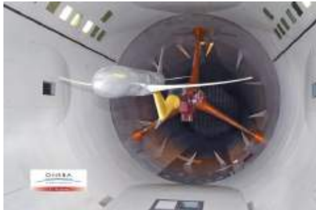
Figure 1: Large Reference Model (LRM) used in the S1-WT at ONERA.
